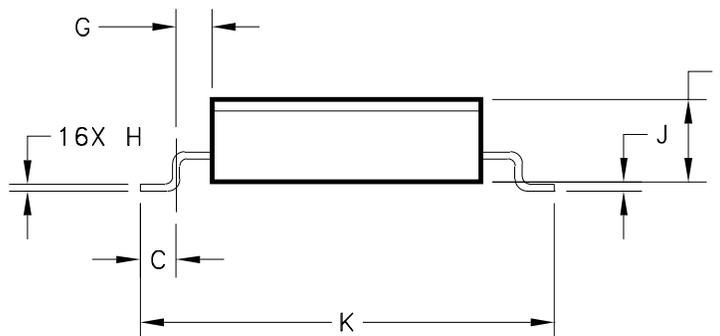
NOTE: "J" IS MEASURED FROM BOTTOM OF PIN TO BOTTOM OF CASE.
