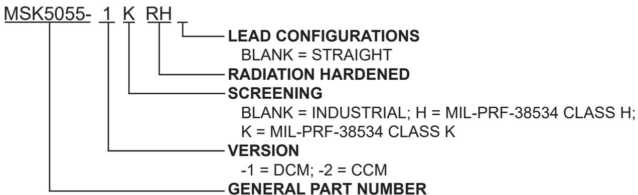
The above example is a DCM, Class K regulator controller with straight leads.
