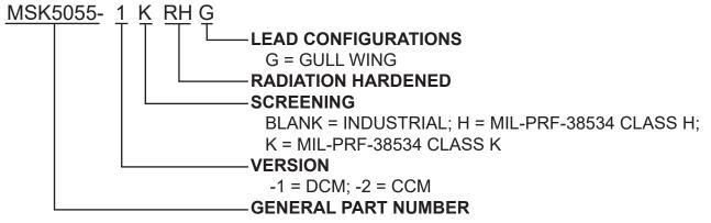
The above example is a DCM, Class K regulator controller with gull wing formed leads.
