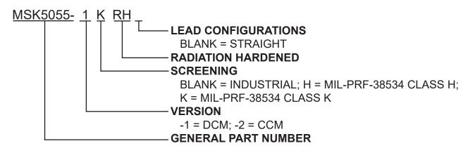
The above example is a DCM, Class K regulator controller with straight leads.
