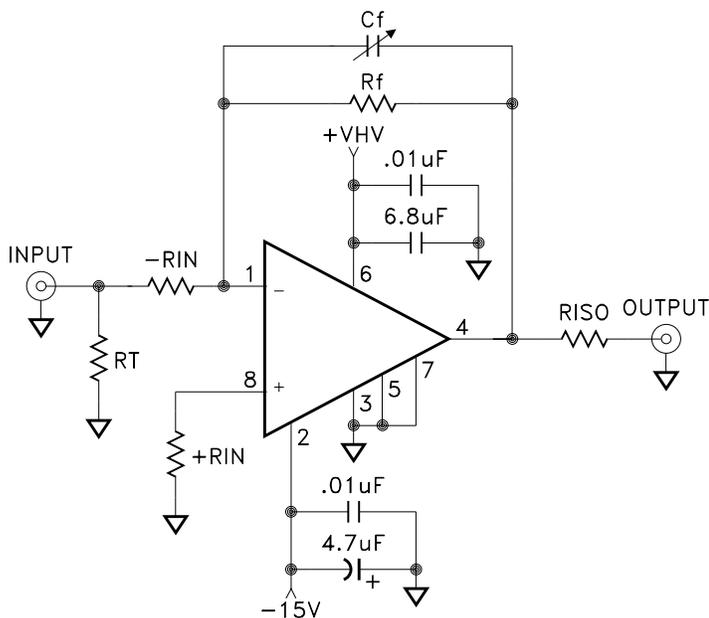
TYPICAL INVERTING CONNECTION DIAGRAM
