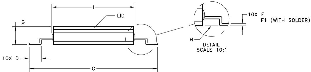
NOTE: LEADS SHALL BE COPLANAR (H) WITH THE PACKAGE BASE.
