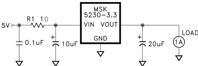
For a given continuous maximum load of 1 amp, R1 can be selected to drop the voltage seen at the regulator to 4V. This allows for the output tolerance and dropout specifications. Input voltage variations (5V) also should be included in the calculations. The resistor should be sized according to the power levels required for the application.
