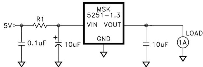
The maximum resistor value can be calculated from the following:
