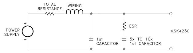
Be careful of the ripple current in all the capacitors. Excessive ripple current, beyond what the capacitors can handle, will destroy the capacitors.
