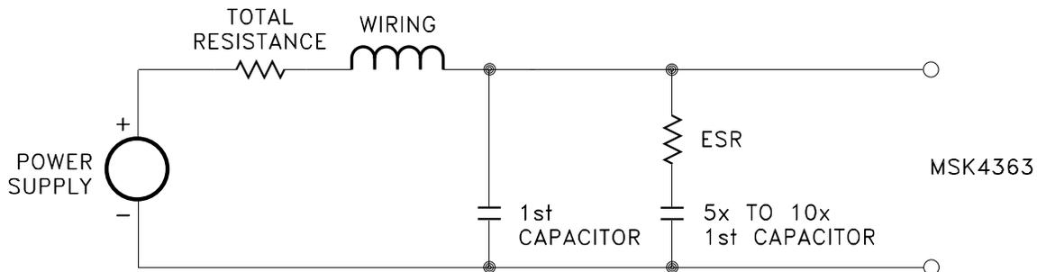
Be careful of the ripple current in all the capacitors. Excessive ripple current, beyond what the capacitors can handle, will destroy the capacitors.
