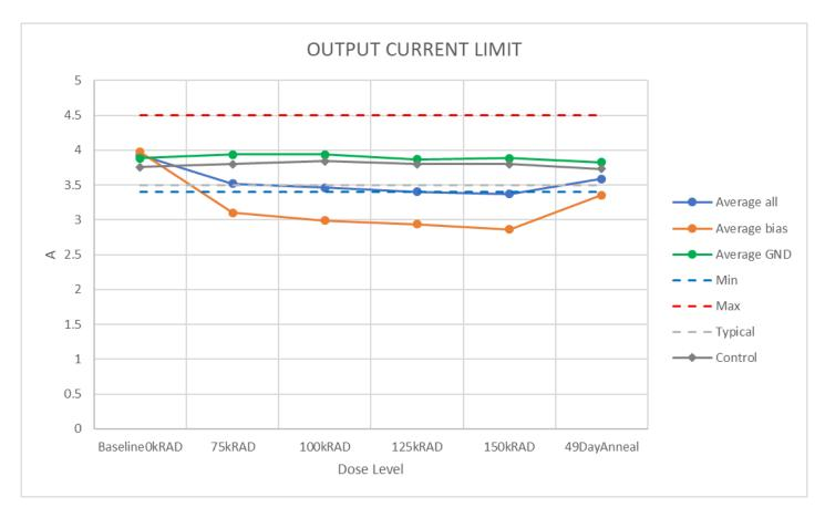
Output Current Limit experienced the largest shift of any parameter, specifically on the Bias devices. This is expected given the HDR TID performance of the regulator IC used in the MSK5065RH and is projected to return to specification within the room temperature anneal time permitted by MIL-STD-883 Method 1019.9.
