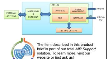
**PLEASE NOTE:** Additional information on the Texas Instruments CC110L device can be found in the company's latest datasheet release at <a href="http://www.ti.com">http://www.ti.com</a>
