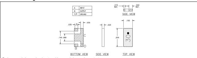
Pad a can only be used as input, pad b can only be used as output
