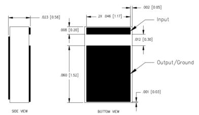
Tolerance is  $\pm 0.004$ ", unless otherwise specified. All dimensions in inches [millimeters].
