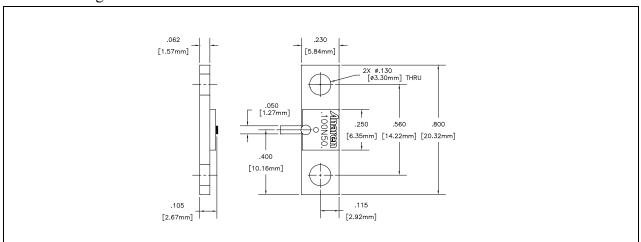
Tolerance is ±0.010", unless otherwise specified. Designed to meet or exceed applicable portions of MIL-E-5400.
