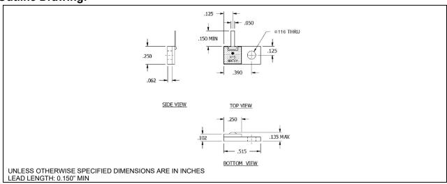
Tolerance is  $\pm 0.010$ ", unless otherwise specified. Designed to meet or exceed applicable portions of MIL-E-5400. All dimensions in inches
