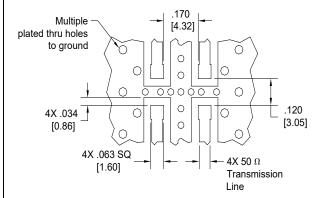
Dimensions are in Inches [Millimeters] 1P510\* Mounting Footprint
