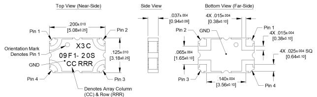
Dimensions are in Inches [Millimeters] X3C09F1-20S Mechanical Outline
