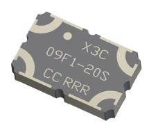
The X3C09F1-20S is a low profile, high performance 20dB directional coupler, with a power rating of 25 W (CW) in a new easy to use, Xinger style manufacturing friendly surface mount package. It is designed particularly for Cellular, 5G & Sub-1GHz Mil-Aero band applications. The X3C09F1-20S is designed for power detection at the outputs of power amplifiers, where low insertion loss and tight amplitude and phase balance is required.
