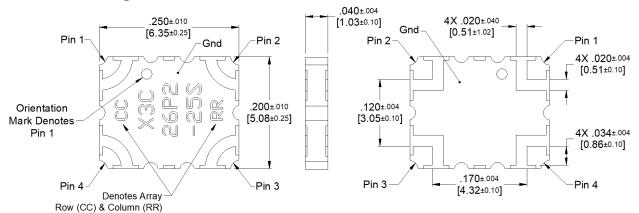
Dimensions are in Inches [Millimeters] X3C26P2-25S Mechanical Outline
