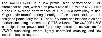
Parts have been subjected to rigorous qualification testing and they are manufactured using materials with coefficients of thermal expansion (CTE) compatible with common substrates such as FR4, G-10, RF-35, RO4003 and polyimide. Produced with 6 of 6 RoHS compliant tin immersion finish.
