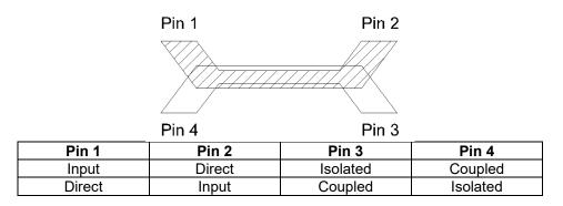
Note: The direct port has a DC connection to the input port and the coupled port has a DC connection to the isolated port. For optimum performance use Pin 1 or Pin 2 as inputs.
