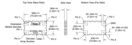
Dimensions are in Inches [Millimeters] XC1900A-05\* Mechanical Outline
