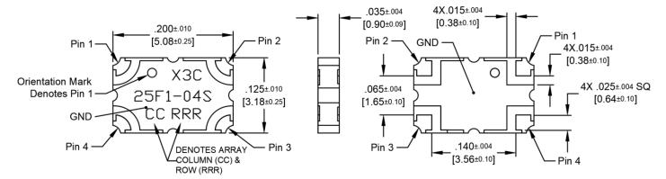
Dimensions are in Inches [Millimeters] X3C25F1-04S Mechanical Outline
