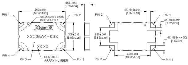
Dimensions are in Inches [Millimeters] X3C06A4-03S Mechanical Outline
