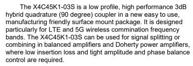
Parts have been subjected to rigorous qualification testing and they are manufactured using materials with coefficients of thermal expansion (CTE) compatible with common substrates such as FR4, RF-35, RO4350 and polyimide. Produced with 6 of 6 RoHS compliant tin immersion finish.
