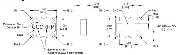
Dimensions are in Inches [Millimeters] Mechanical Outline
