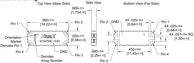
Dimensions are in Inches [Millimeters] XC0450E-03S Mechanical Outline
