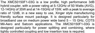
Parts have been subjected to rigorous Xinger qualification testing and they are manufactured using materials with coefficients of thermal expansion (CTE) compatible with common substrates such as FR4, G-10, RF-35, RO4350 and polyimide. Available in ENIG RoHS compliant finish.
