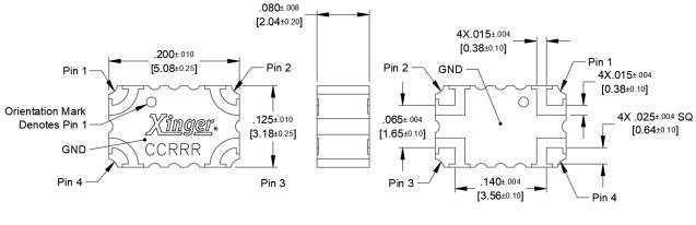
Dimensions are in Inches [Millimeters] XMC50150F1-03G Mechanical Outline
