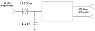
Note: The performance below is shown with series Resistor R1 of 10 Ohms and parallel capacitor C1 of 1.1pF tuned at pin 1 (50 Ohm port).
