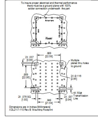
In order for Xinger surface mount delay lines to work optimally, there must be  $50\Omega$  transmission lines leading to and from all of the RF ports. Also, there must be a very good ground plane under the part with a number of plated thru holes to insure proper electrical performance. If any of these conditions are not satisfied, insertion loss, average delay and VSWR may not meet published specifications.
