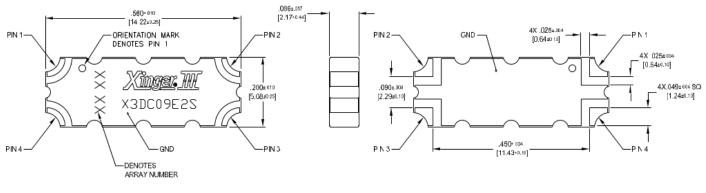
Dimensions are in Inches [Millimeters] X3DC09E2S Mechanical Outline Tolerances are Non-Cumulative
