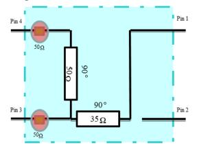
The X3DC09E2S has an orientation marker to denote Pin 1. Once port one has been identified the other ports are known automatically. Please see the chart below for clarification:
