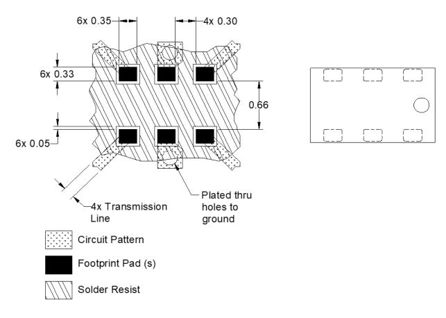
Dimensions are in Millimeters Mounting Footprint
