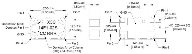
Dimensions are in Inches [Millimeters] X3C14F1-02S Mechanical Outline
