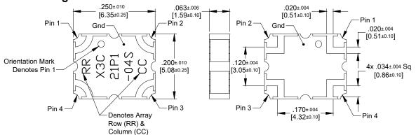
Dimensions are in Inches [Millimeters] X3C21P1-04S Mechanical Outline
