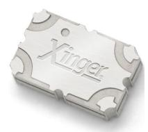
The X3C25F1-02S is a low profile, high performance 2dB hybrid coupler in a new easy to use, manufacturing friendly surface mount package. The X3C25F1-02S is designed particularly for balanced power and low noise amplifiers, plus signal distribution and other applications where low insertion loss and tight amplitude and phase balance is required. It can be used in high power applications up to 20 watts.
