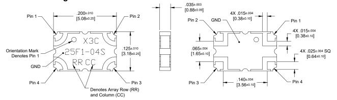
Dimensions are in Inches [Millimeters] X3C25F1-04S Mechanical Outline
