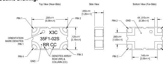
Dimensions are in Inches [Millimeters] X3C35F1-02S Mechanical Outline Tolerances are Non-Cumulative
