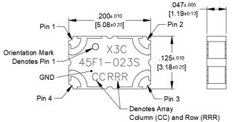
Dimensions are in Inches [Millimeters] X3C45F1-023S Mechanical Outline
