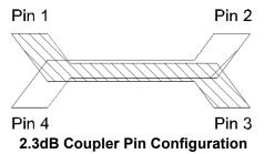
Configuration Pin 2 Pin 3 Pin 1 Pin 4 **Splitter** Isolated Input  $-4dB < \Theta - 90$ -2.3dB < ⊖ **Splitter** Isolated Input  $-4dB < \Theta - 90$ -2.3dB  $< \Theta$ **Splitter** Input Isolated -2.3dB < ⊖  $-4dB < \Theta - 90$ **Splitter** Isolated Input -2.3dB < ⊖  $-4dB < \Theta - 90$
