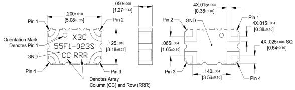
Dimensions are in Inches [Millimeters] X3C55F1-023S Mechanical Outline
