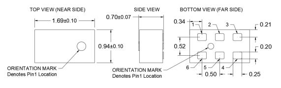
Dimensions are in Millimeters Tolerance are Non-Cumulative
