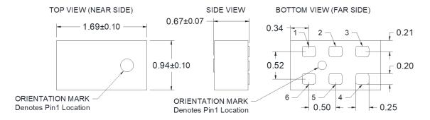
Dimensions are in Millimeters
