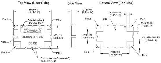
Dimensions are in Inches [Millimeters] XC0450A-03S Mechanical Outline
