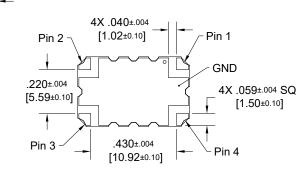
Dimensions are in Inches [Millimeters] \* For RoHS Compliant Versions order with S suffix XC0900A-05\* Mechanical Outline
