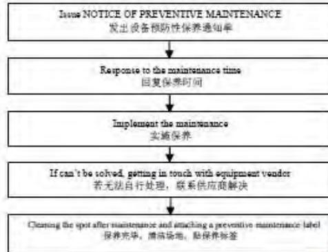
Fig 2. Equipment breakdown repair flow chart 图2.设备维修流程图
